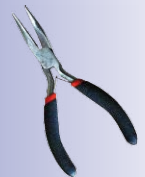
Pliers to break through a cable guide
